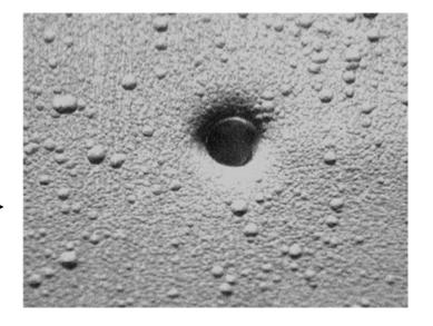
2<sup>nd</sup> Generation PFOS free surfactants provide better solubility preventing formation of pores at high levels of metal contamination in the Chrome solution
