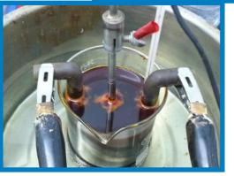
Lab simulation at identical conditions, 55°C, 10 A, 50 A/dm<sup>2</sup>, 900 ml, 1h, 33 Dyne/cm
