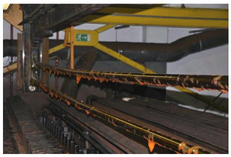
2<sup>nd</sup> Generation PFOS-free Foamless at 30 Dyne/cm No risk of H<sub>2</sub> explosions Low consumption rate Cooling effect of evaporation remains 1<sup>st</sup> Generation PFOS-free Strong formation of foam at 35 Dyne/cm Risk of H<sub>2</sub> explosions High drag out rate/consumption High demand for cooling
