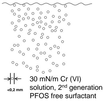
•Bigger diameter bubbles bring more kinetic energy with them to the surface of the solution compared to smaller bubbles.
